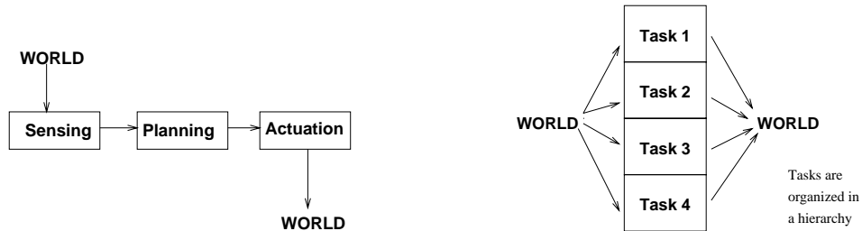
Figure 3: Traditional vs. Reactive . Reactive robots are based on behaviors that mediate directly with the outside world and communicate very little between themselves.
