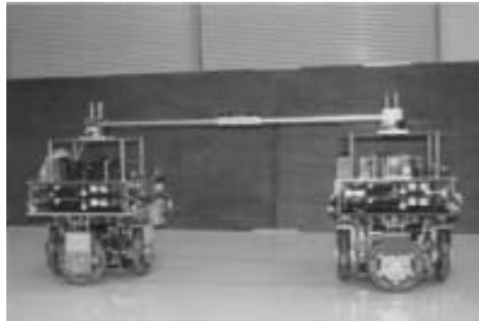
Figure 1: RIKEN’s omni-directional robots carrying a bar (ladder).
